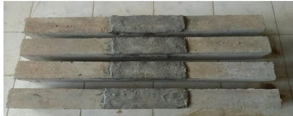
Fig. 3 Beams retrofitted using cement matrix composite
